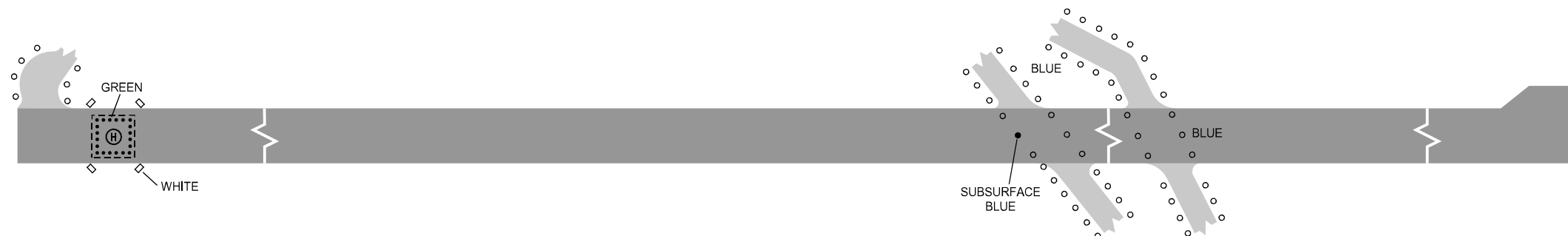
LIGHTING AIDS RWY 05L / 23R AND EXIT TWY
